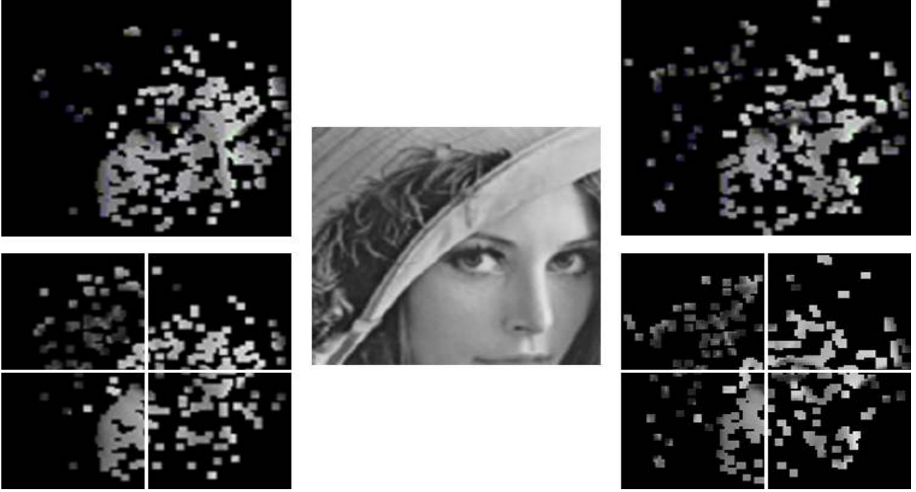
Figure 1. Linear and quadratic subsets learned for a sample template. The top left template shows the linear subsets used with the inverse compositional algorithm and the top right template shows the quadratic subsets used with the ESM algorithm. The bottom row shows the linear and quadratic subsets obtained when the subsets are constrained to be spread evenly over the template. Building such subsets takes less than 30 seconds on a standard computer.
