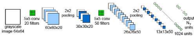
Fig. 5. Architecture of the CNN \text{CNN}^{\text{cp-pred-p}} predicting the projections of the control points.
