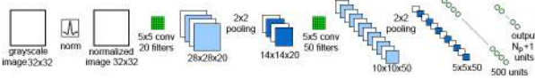
Fig. 4. Architecture of \text{CNN}_{\text{part-det}} for part detection. The last layer outputs the likelihoods of the patch to correspond to each part or to the background.
