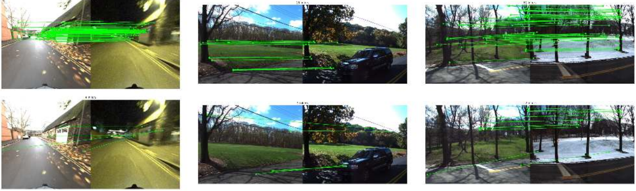
Figure 4: Examples of inlier correspondences obtained using RANSAC+PnP. Top-row shows correspondences obtained with our method, bottom row shows correspondences obtained with SuperPoint detection and descriptors.
