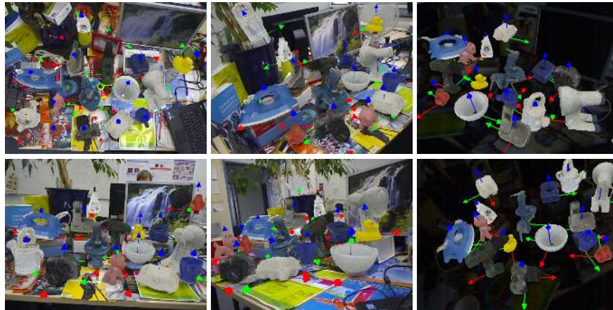
Fig. 3. 15 different texture-less 3D objects are simultaneously detected under different poses on heavy cluttered background with partial occlusion and illumination changes. Each detected object is augmented with its 3D model and its coordinate systems.
