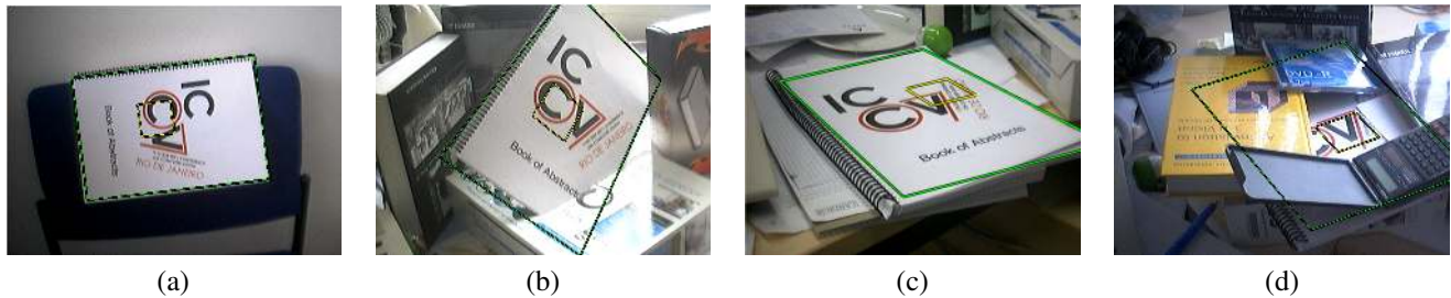
Figure 9. Accuracy of the retrieved transformation. For each of these images, we draw the borders of the book estimated from a single patch. This is made possible by the fact we estimate a full perspective transform instead of only an affine one.
