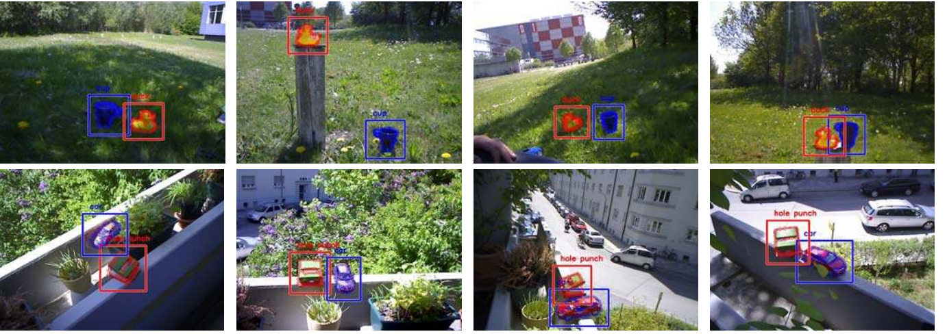
Fig. 14: Different texture-less 3D objects are detected with LINE-2D in real-time under different poses in difficult outdoor scenes with partial occlusion, illumination changes and strong background clutter.
