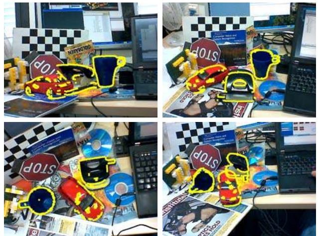
Fig. 1: Our method can detect texture-less 3D objects in real-time under different poses over heavily cluttered background using gradient orientation.
