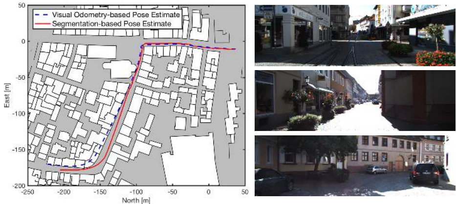
Figure 6: Trajectory estimated via visual odometry (dotted blue line) and the corrected trajectory using our segmentation-based tracking (solid red line) (left). Illustrative examples from KITTI Sequence #18 showing highly over- or underexposed façade areas (right).
