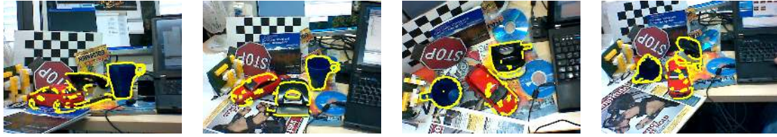
Figure 6.1: Our method can detect texture-less 3D objects in real-time under different poses over heavily cluttered background using gradient orientation.
