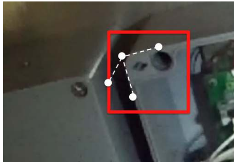
Figure 8.2: Detecting and estimating the pose of the box from Fig. 8.1(a). We propose to first detect discriminative parts, such as the visible corners, and predict the 3D orientation of each part. The part 3D orientation can be parameterised by control points, represented here with white dots.
