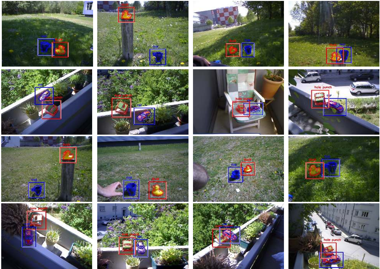
Figure 6.13: Different texture-less 3D objects are detected with LINE-2D in real-time under different poses in difficult outside scenes with partial occlusion, illumination changes and strong background clutter.
