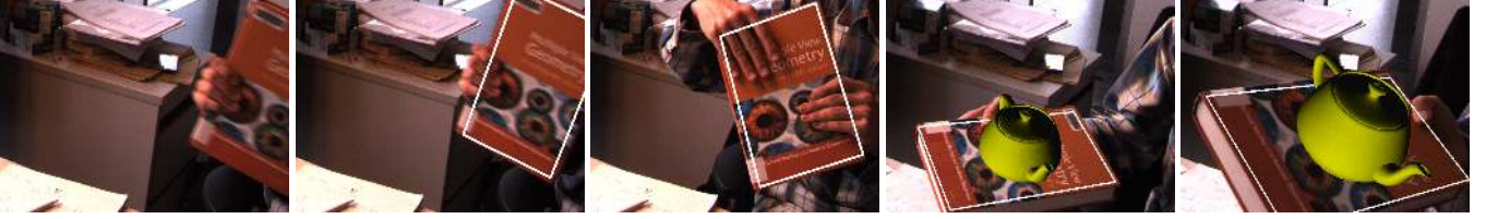
Figure 1. The advantages of tracking-by-detection approaches for Augmented Reality. The target object, the book in this example, is detected in every frame independently. No initialization is required from the user, and tracking is robust to fast motion and complete occlusion. The objects 3D pose can be estimated and the object can be augmented.
