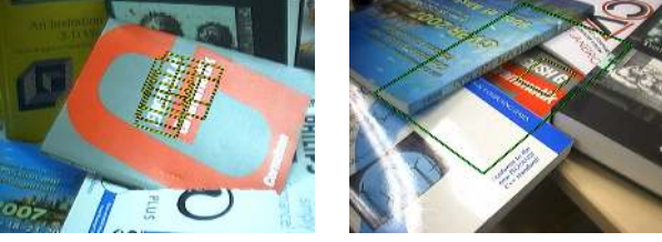
Figure 2. Relaxing the need for texture. [1] not only matches feature points, but also estimates their local pose. These local poses can be extended to retrieve the object pose. As a result, a single feature is often enough to make the method very robust to occlusion (right image), and suitable for low textured objects.
