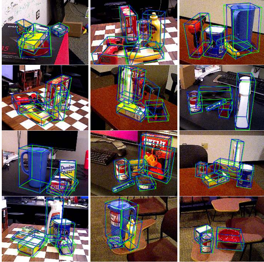
Fig. 5: Qualitative results on the YCB-Video dataset [2]. We show the 3D bounding boxes of the objects projected to the color image. Ground truth poses are shown in green, our predictions are shown in blue.
