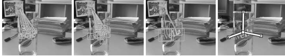
Fig. 7. Detecting a transparent object with partial texture. The squares in the first three images outline the patches around the features detected at three different scales in a test frame. The straight line segments connect the feature with the corresponding one in a frame of the training sequence. Since during training the system learned which parts of the patches are meaningful as shown in Fig. 3, the image features can be recognized even if the patch overlaps the background or the transparent parts. As shown in the fourth frame, the glass is successfully detected.
