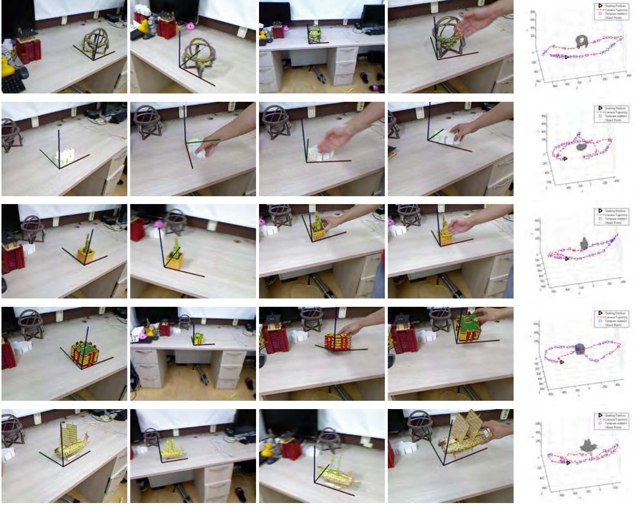
Figure 5: Tracking of various objects. First row: A hon-chun-eui (an old armillary sphere in Korea); Second row: A miniature building; Third row: A cactus; Fourth row: Another miniature Building; Fifth row: A toy ship. The poses are correctly estimated under various viewpoints, partial occlusions, and fast motion. The rightmost column shows the estimated trajectory of the camera with respect to the object; For visibility, we show only the training part. The complete sequences are available in the supplementary video.
