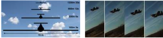
Figure 9: Collision courses. (Left) The apparent size of a standard glider and its 15 m wingspan flying towards another aircraft at a relatively slow speed (100 km/h) is very small 33s before impact, but the glider completely fills the field of view only half a minute later, 3s before impact. (Right) An aircraft on a collision course is seen in a constant direction but its apparent size grows, slowly at first and then faster.
