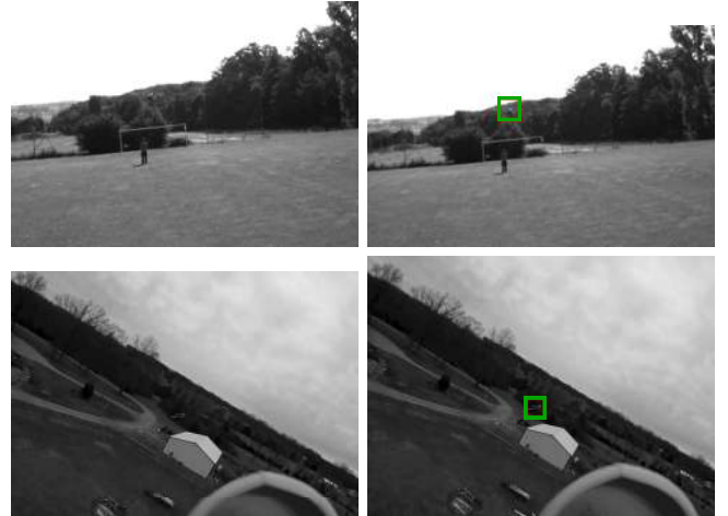
Figure 1: Detecting a small flying object against a complex moving background. (Left) It is almost invisible to the human eye and hard to detect from a single image. (Right) Yet, our algorithm can find it by using appearance and motion cues.
