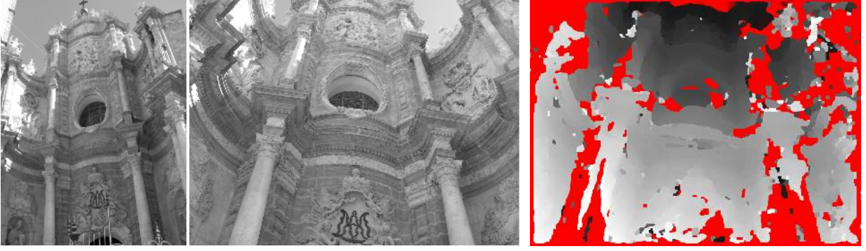
Figure 18. Valencia Cathedral. The reconstruction results of the exterior of the Valencia Cathedral from two very different viewpoints. Depth map is computed from the 2 nd image's point of view.
