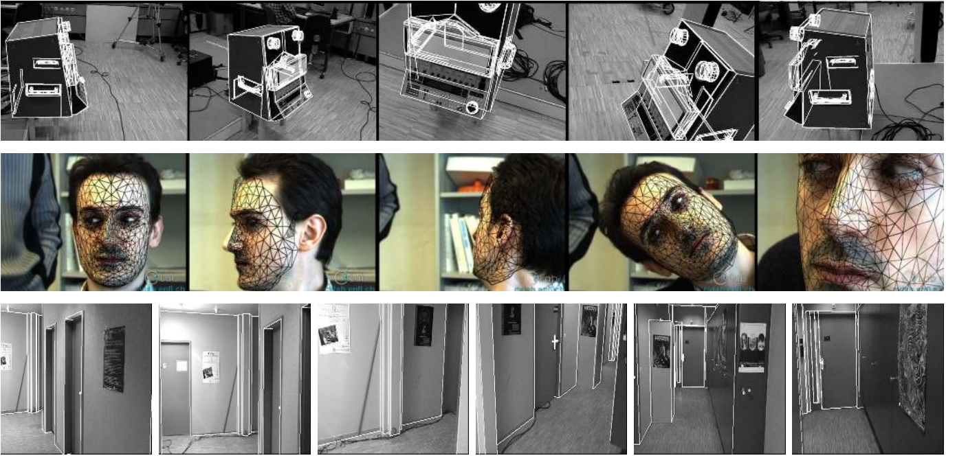
Fig. 1. First row: Video sequence with overlaid 3D model whose pose has been computed online using eight keyframes. Second row: We track a face using a generic model that has not been tailored for this specific man using one keyframe. Third row: The same method is used to track a 1000 frames video sequence of a corridor. We used four keyframes. The corresponding video sequences are submitted as supplementary material.
